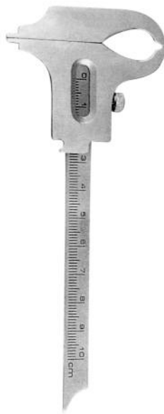
Fig.2 QI-08-194 Boley Measuring range 0-100 mm
